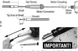
loosening the set screw in the motor connector and moving the sheath in or out while the motor and shaft/sheath are hanging fully extended or laying on a flat surface. When the shaft is adjusted correctly, tighten the set screw in the motor connector.
